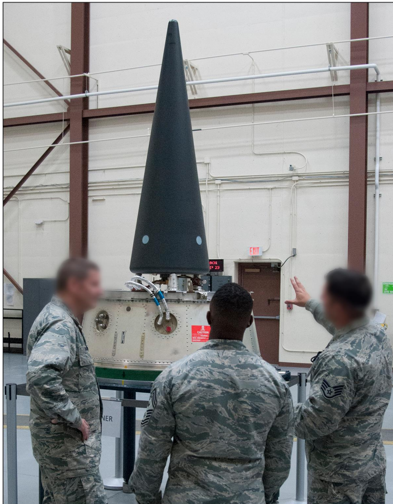
Figure 2: W87-0 Warhead Contained within a Mk21 Reentry Vehicle
