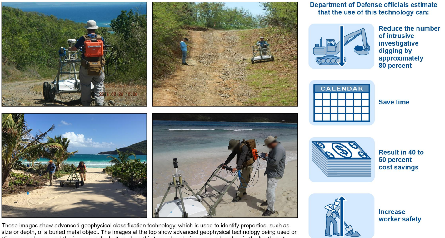
Figure 9: Advanced Geophysical Classification Technology Used at Cleanup Sites on Vieques and Culebra, Puerto Rico
