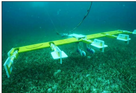
Detection of potential munitions is done by measuring and recording magnetic anomalies caused by the presence of iron objects lying on or beneath the seafloor.
