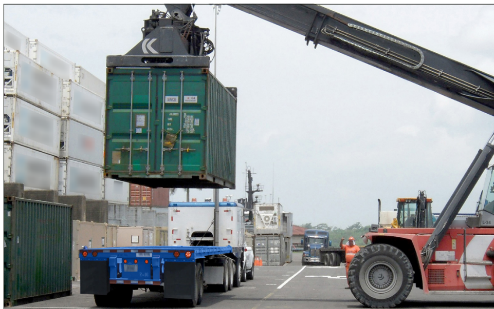
Figure 1: A Shipping Container Being Placed on an Intermodal Chassis
