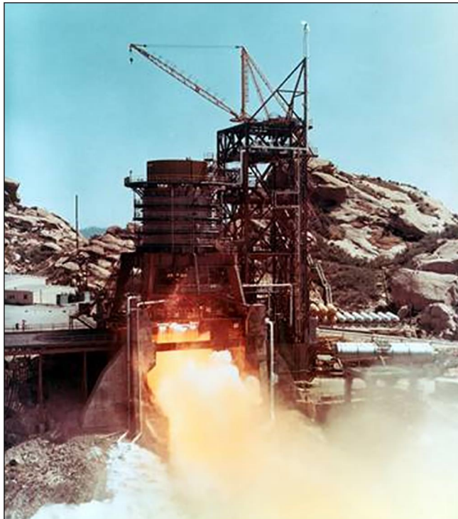
Figure 2: Rocket Engine Testing at NASA's Santa Susana Field Laboratory in 1965
