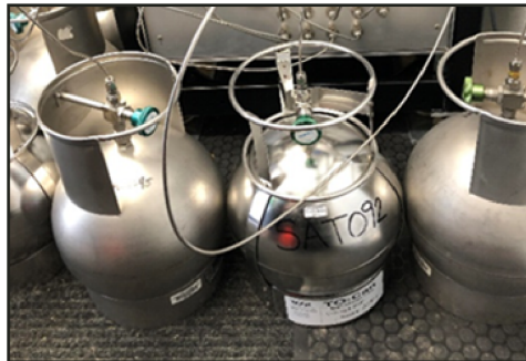
Canisters used to collect samples for measuring air toxics operated by the Wisconsin Department of Natural Resources
