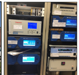
Equipment for monitoring criteria pollutants operated by the Colorado Department of Public Health and Environment
