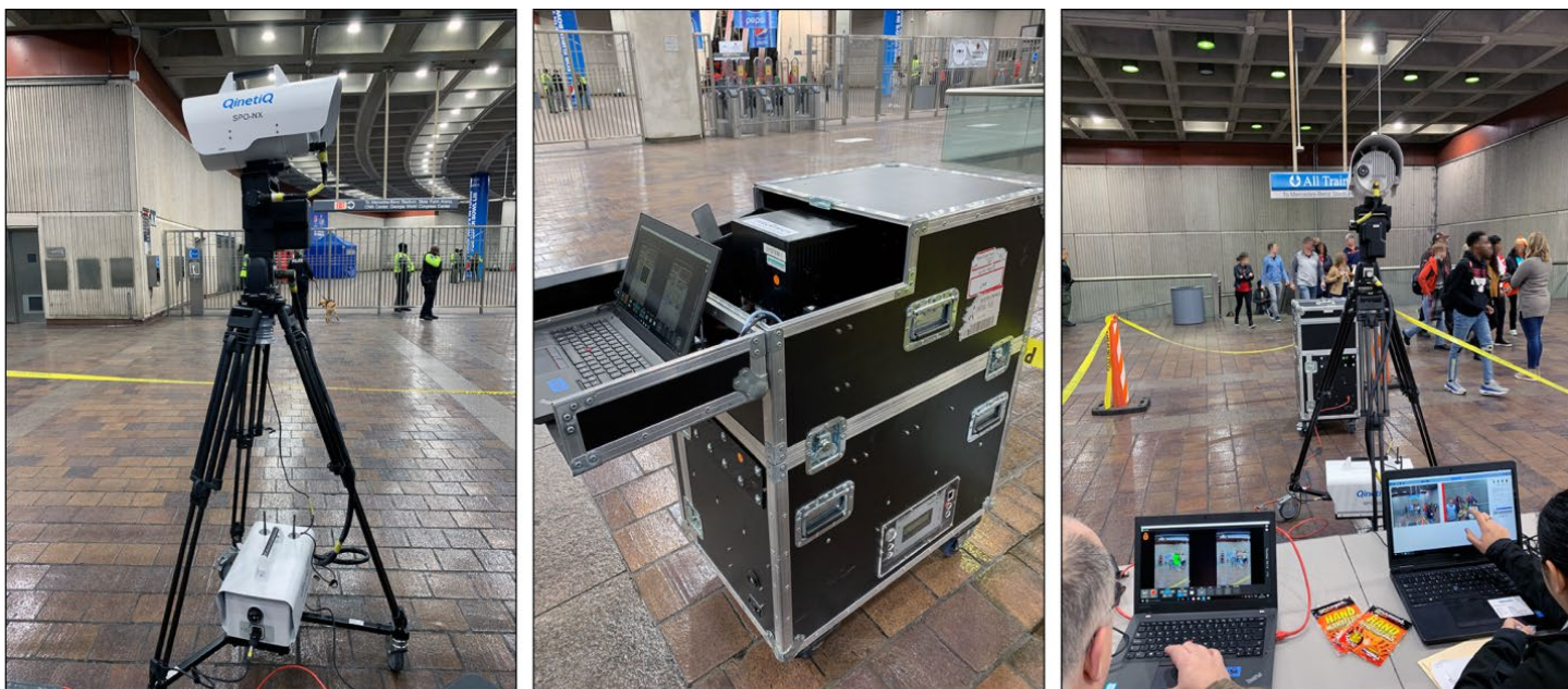
Both the QinetiQ SPO-NX (left) and ThruVision TAC (middle) technologies were used to scan passengers for anomalies and explosives (right).
