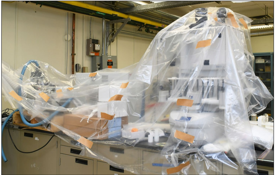
Figure 5: Equipment Covered to Protect It from Rainwater in the Analytics and Chemistry Laboratory at the Pantex Plant
