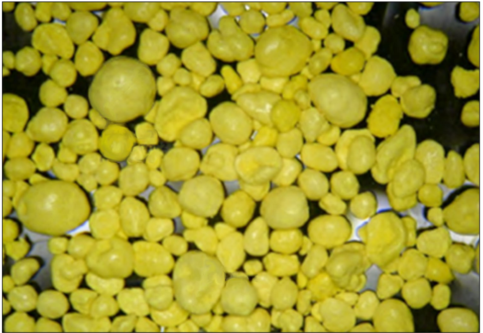
Figure 3: Formulated High Explosive Prills (Irregularly Shaped Pebbles)
