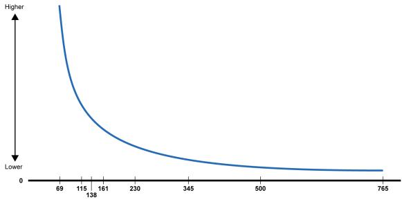
Resistance (transmission line direct current resistance per unit distance)
