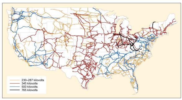
Figure 11: High-voltage electric transmission lines in the contiguous United States by voltage class
