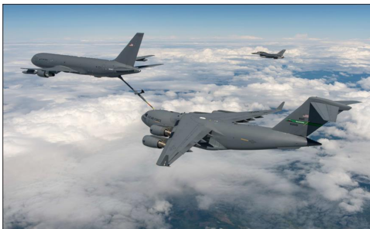
Figure 1: KC-46 Aircraft Using the Boom to Refuel a Receiver Aircraft
