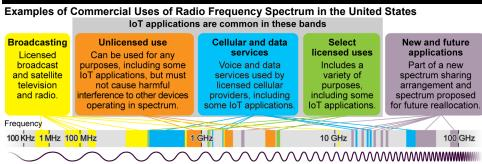
Lower frequencies have longer wavelengths, which carry small amounts of data but are able to penetrate dense objects. Source: GAO analysis. | GAO-18-71
