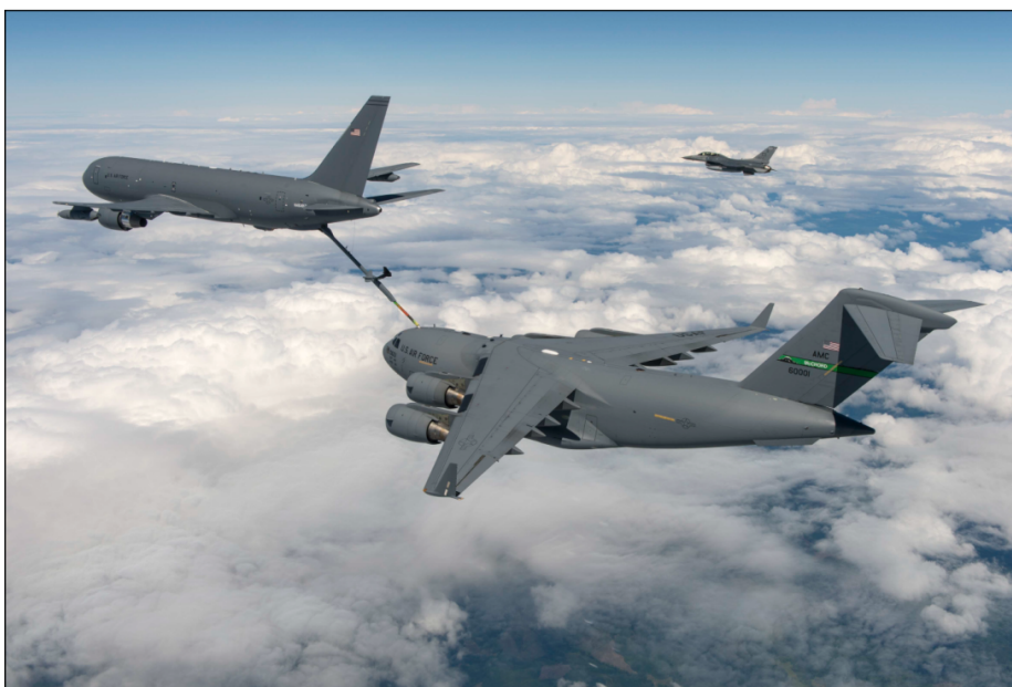
Figure 1: KC-46 Aircraft Using the Boom to Refuel a Receiver Aircraft
