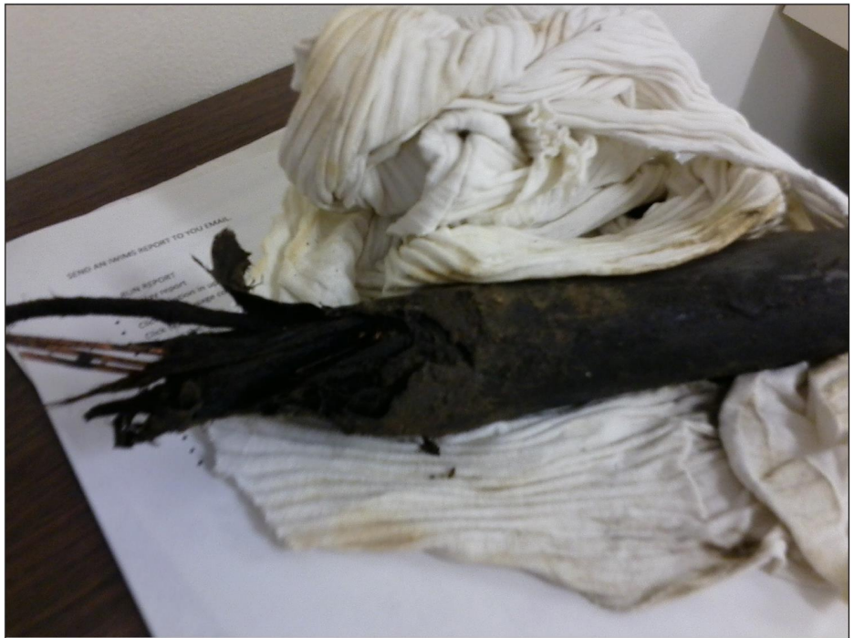
Figure 5: Burnt Electrical Feeder Cable That Caused a Major Disruption to an Army Facility on Joint Base McGuire-Dix-Lakehurst, New Jersey
