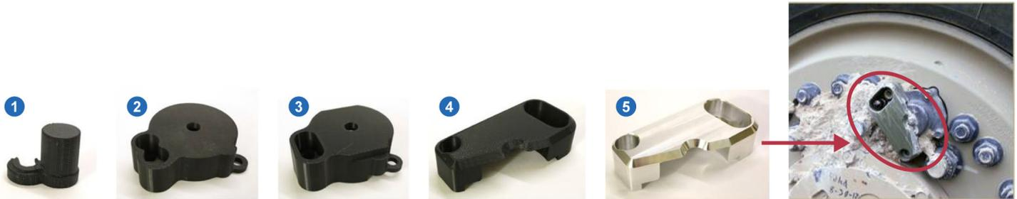
The Army additively manufactured versions 1 through 4 of the covers before a final part was produced through conventional manufacturing (shown in version 5).
