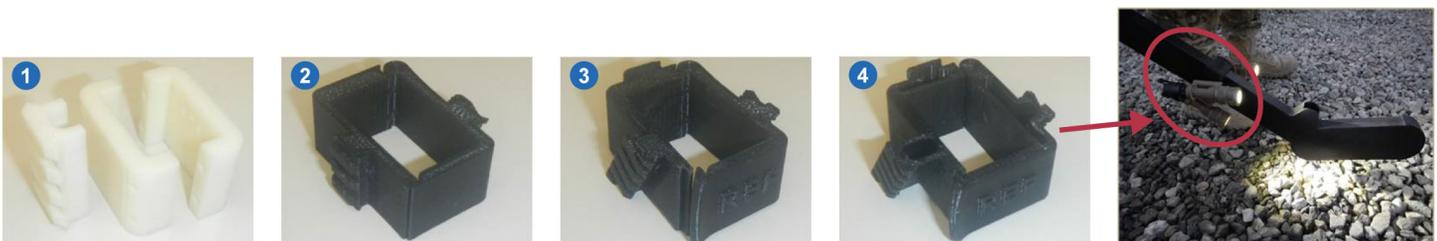
The Army additively manufactured mounting brackets for attaching flashlights to mine detectors in four versions.
