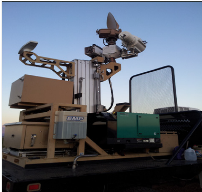
Figure 1: Mobile Surveillance System Imager/Radar Upgrade –A Retrofit Kit Developed by S&T BMD for CBP Tested at the Arizona-Mexico Border
