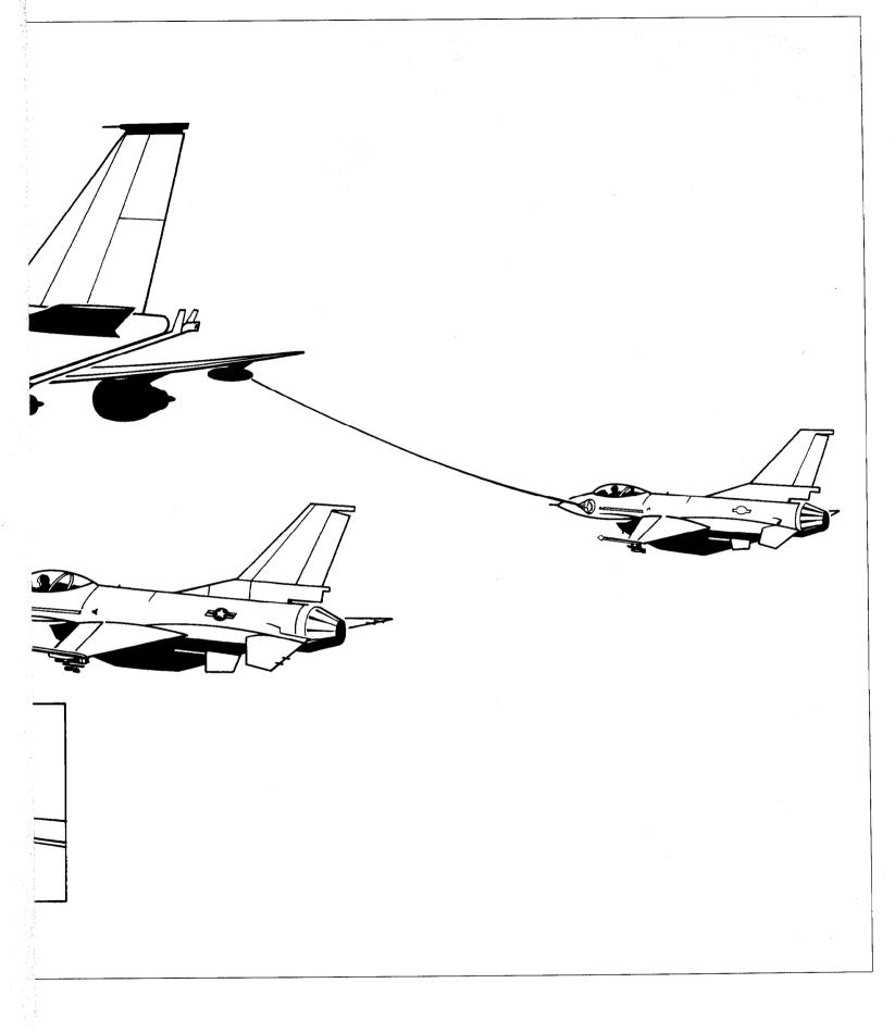
In contrast, Air Force fighters refuel with a boom/receptacle system. The boom is a telescoping tube mounted near the tail of a tanker. During refueling, the boom operator aboard the tanker maneuvers the tip of this tube into a receptacle aboard the receiver aircraft (see fig. 2).
