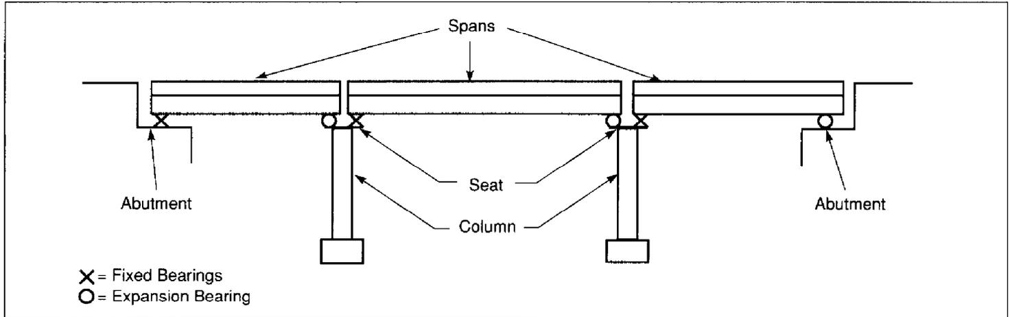
A common reason for damage in simply supported bridges is inadequate seatwidths of the girder supports. During shaking, large relative movements between the girder and the support can unseat the girder, which could damage or cause the collapse of one or more bridge spans (see fig. II.4).
