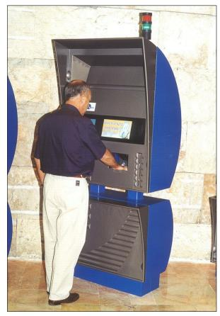
Figure 34: A Traveler Using Ben Gurion Airport's Biometric Hand Geometry System
