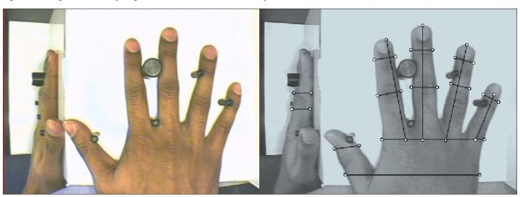
Figure 32: Fingers Guided by Pegs in a Biometric Hand Geometry Measurement
