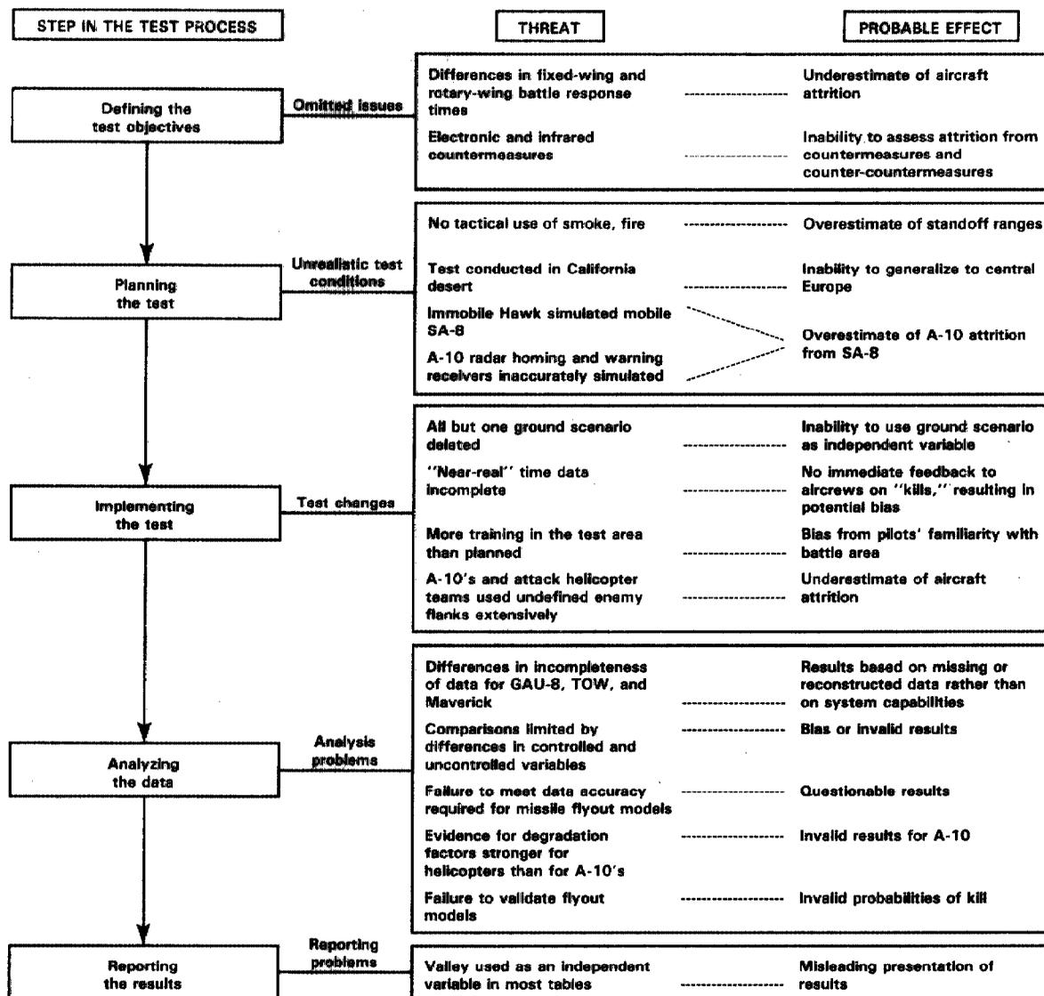
The effect of countermeasures on combat was dropped as a test objective. No electronic or infrared countermeasures were used. Thus, the interaction of countermeasures and counter-countermeasures was not tested. If it had been tested, the tactics for friendly air forces and enemy air defense units, and the attrition results, might have been different.
