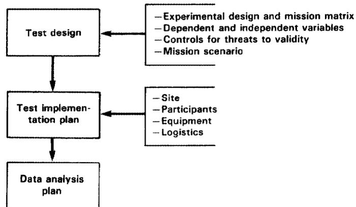
As figure 12 shows, the decisions may take the form of a test design, a test implementation plan, and a data analysis plan.
