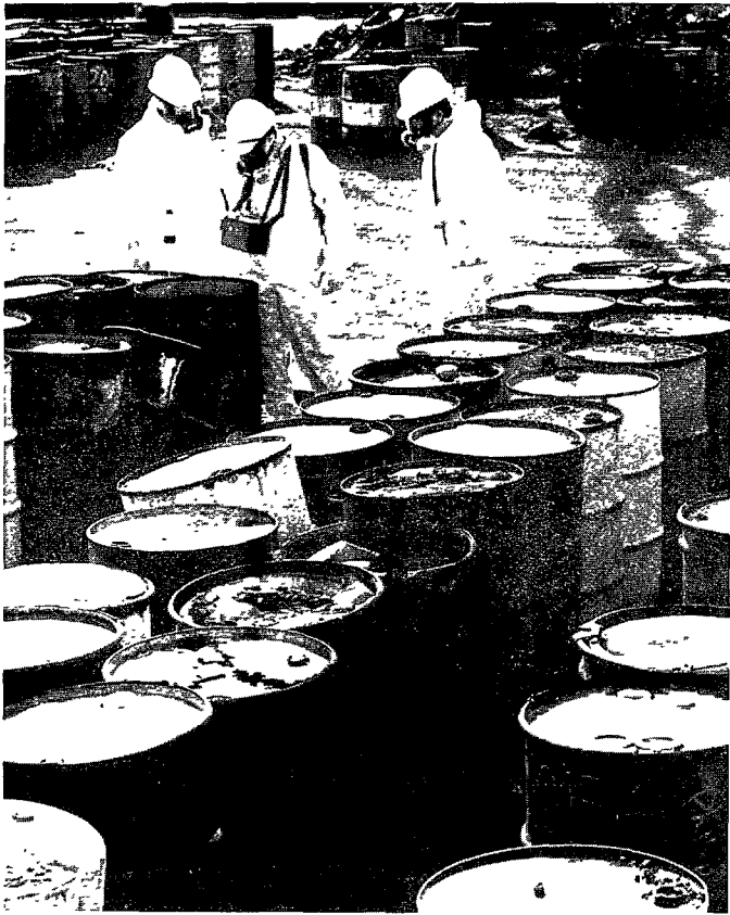
Hazardous wastes are sampled and tested prior to cleanup at the Chem-Dyne site in Ohio.
