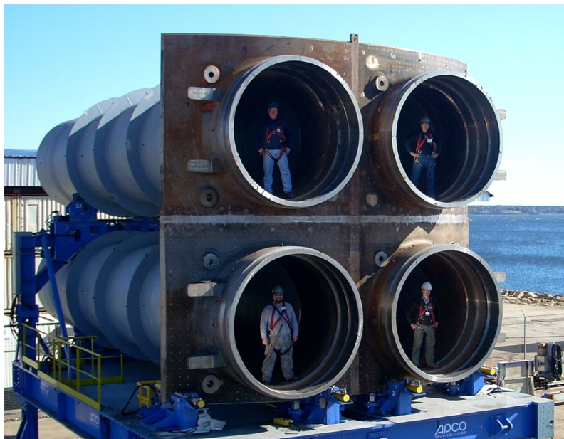
Quad Pack of Four Submarine Missile Tubes
