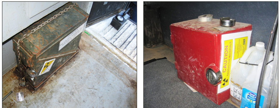
Figure 5: Radiography Camera Box Padlocked within Its Cradle and High-Security Box Bolted to the Floor of the Truck
