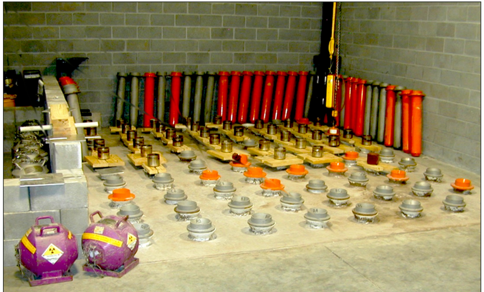
Figure 9: Well Logging Storage Facility with Multiple Containers for Storing Radiological Sources
