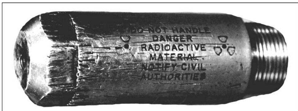
Figure 2: Example of a Radioactive Sealed Source That Contains Americium-241
