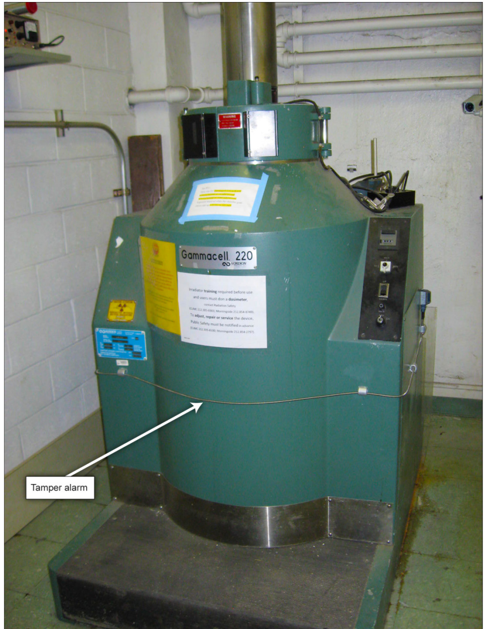
Figure 8: Irradiator with NNSA-Installed Tamper Alarm around Middle of Device
