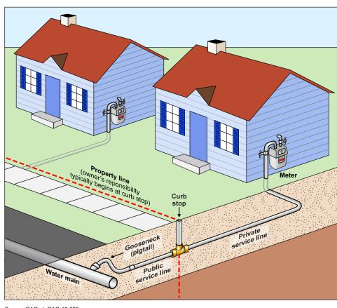
Figure 1: Typical Location of Water Main, Lead Service Line, and Other Pipes That Deliver Drinking Water to Homes
