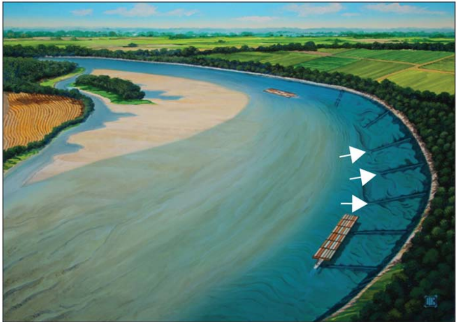
Figure 4: Illustration of Submerged Bendway Weirs on the Outside of a River Bend
