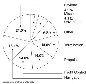
Figure 4: JASSM Subsystems Involved in Flight Test Failures
