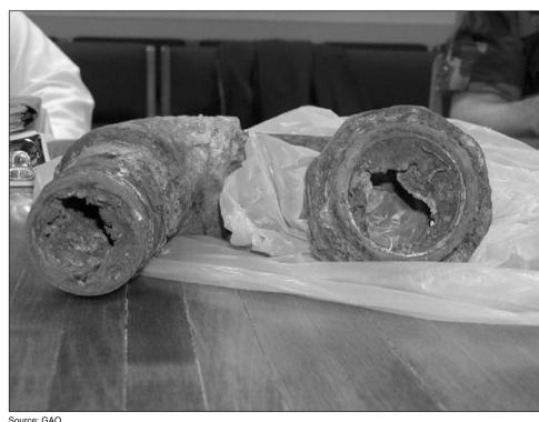
Figure 6: Choked and Clogged Water Pipes at Pope Air Force Base, North Carolina
