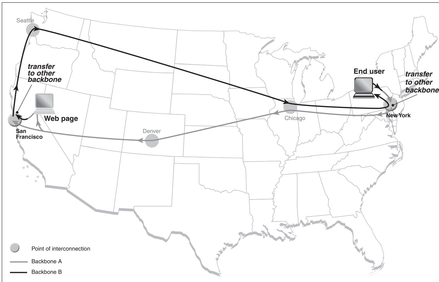
Figure 4: Routing of Internet Traffic Among Comparably Sized Backbone Providers
