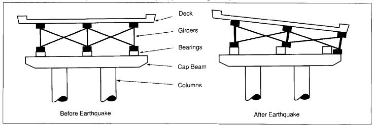
The Fields Landing Overhead collapse near Eureka, California was caused principally by the inadequate length of the seatwidths supporting the bearings which resulted in the bridge spans slipping off their supports (see fig. II.5).
