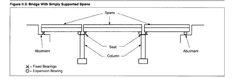
A common reason for damage in simply supported bridges is inadequate seatwidths of the girder supports. During shaking, large relative movements between the girder and the support can unseat the girder, which could damage or cause the collapse of one or more bridge spans (see fig. II.4).
