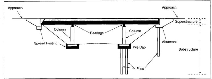
Figure II.1: Common Bridge Components
