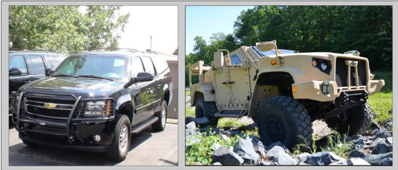
Figure 1: Typical Armored Commercial Passenger-Carrying Vehicle (left) Compared with Tactical Vehicle (right)
