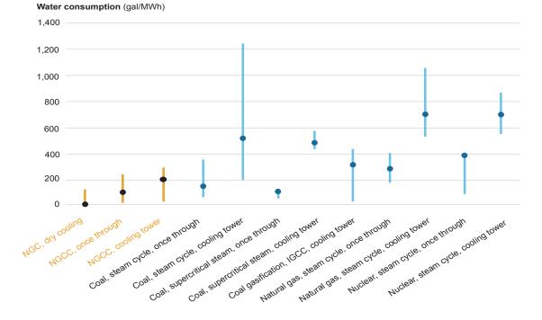
**Figure 5.6**: Estimates of water consumption by various thermoelectric plant types and cooling systems Source: GAO analysis of Meldrum et al. 2013 and National Renewable Energy Laboratory 2011 | GAO-15-545 Notes: NGCC denotes natural gas combined cycle; IGCC denotes integrated gasification combined cycle. The data points indicate median values while the error bars show the extent of variability of water consumption in the given data set.
