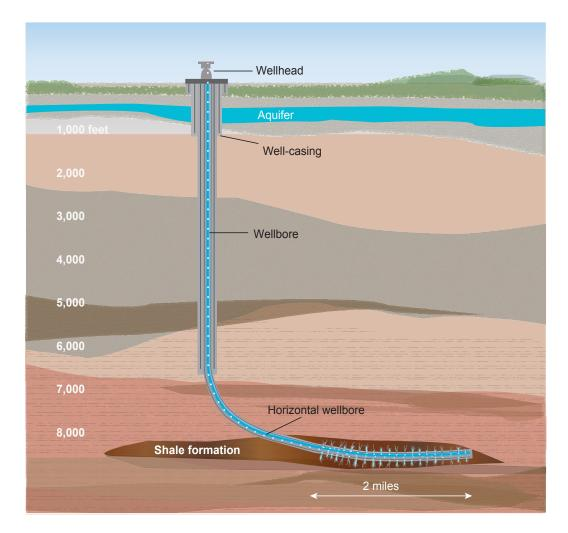
Figure 2.3: A horizontally drilled, hydraulically fractured shale gas well Source: GAO adapted from Argonne National Laboratory 2012 | GAO-15-545
