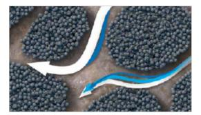
Figure 3.2: Flow channel creation with channel fracturing technology
