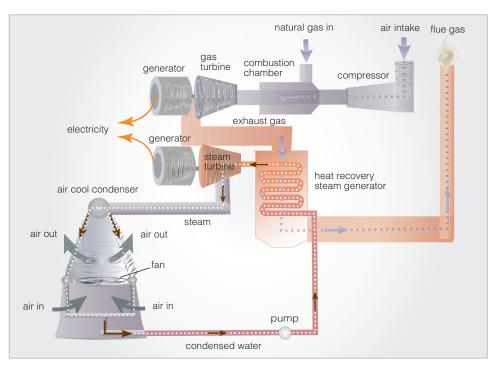
A natural gas combined cycle (NGCC) power plant with a dry cooling system. Source: GAO. | GAO-15-545
