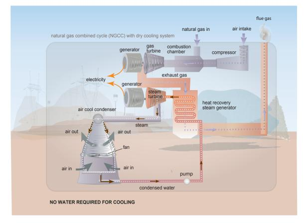
**Figure 4.2**: A natural gas combined cycle (NGCC) power plant with a dry cooling system Source: GAO adaptation of GAO 2009a and Electric Power Research Institute 2008 | GAO-15-545
