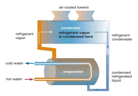
Figure 7.2: Thermosyphon cooling technology Source: GAO, adapted from Electric Power Research Institute 2012e and Johnson Controls | GAO-15-545
