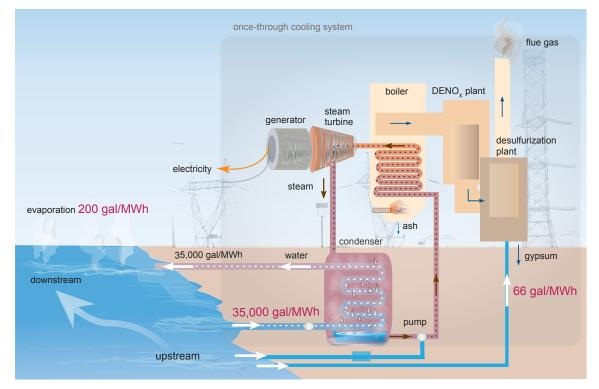
Figure 2.5: A coal power plant with a once-through cooling system Source: GAO adaptation of Electric Power Research Institute 2013, U.S Department of Energy 2007, and Meldrum et al. 2013 | GAO-15-545
