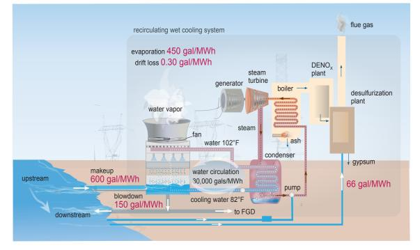
**Figure 2.6**: A coal power plant with a wet recirculating cooling system Source: GAO adaptation of Electric Power Research Institute 2013a and National Energy Technology Laboratory 2007c | GAO-15-545
