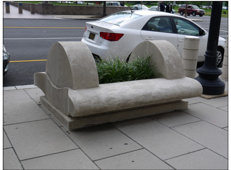
Security bollard that also serves as a bench and planter
