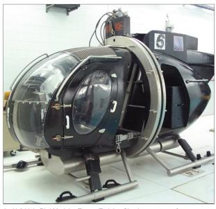
An H-6 Little Bird Modular Egress Training Simulator, a type of egress simulator used by Special Operations Command to train its Little Bird pilots, aircrew, and passengers on a replica of their specific airframe.
