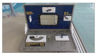
A Shallow Water Initial Memory Mechanical Exit Release device, a type of problem-solving trainer used by the Navy to teach students to operate helicopter exit release controls underwater and develop their confidence prior to training in its egress simulators.
