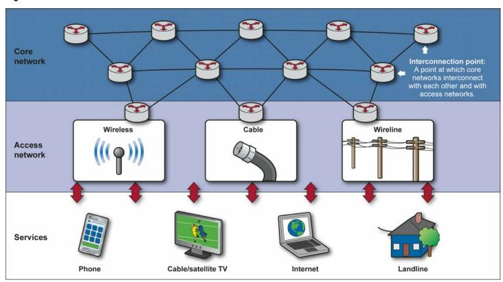
Figure 1: Communications Core and Access Networks
