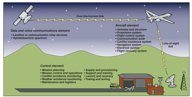
Figure 1: Conceptual Rendering of Unmanned Aircraft System
