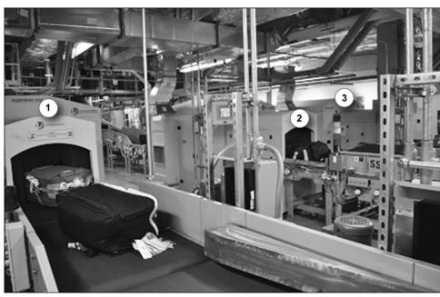
Figure 3: A Checked Baggage Inspection System That Includes a Baggage Handling System with Three In-line EDS Machines
