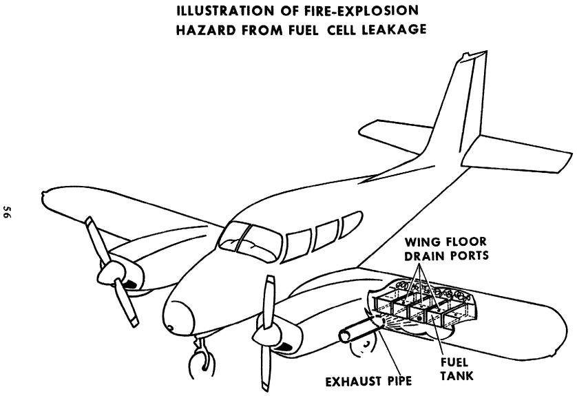
FAA issued General Aviation Inspection Aids<sup>1</sup> which cited the fuel leakage problem and which recommended that fuel tanks be kept full when the aircraft were not in operation.
