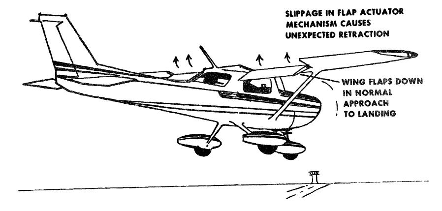
at the time these aircraft were certified, clearly stated that flaps had to be designed so that they would not slip. Records of Cessna-type certification ground and flight tests indicated no problem with the flap actuator.
