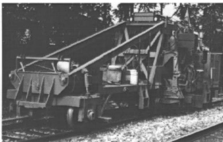
Tamper/liner, used to smooth the surface of the ballast and align the track.
